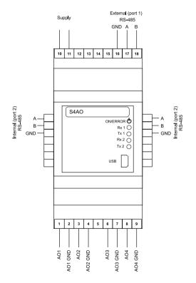
Figure 3: Electrical connections of the S4AO module.
