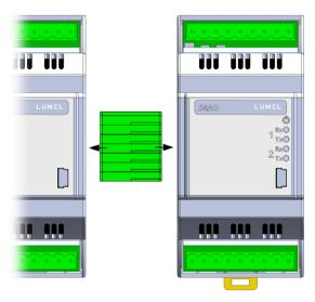
Figure 6: lateral bus connection
